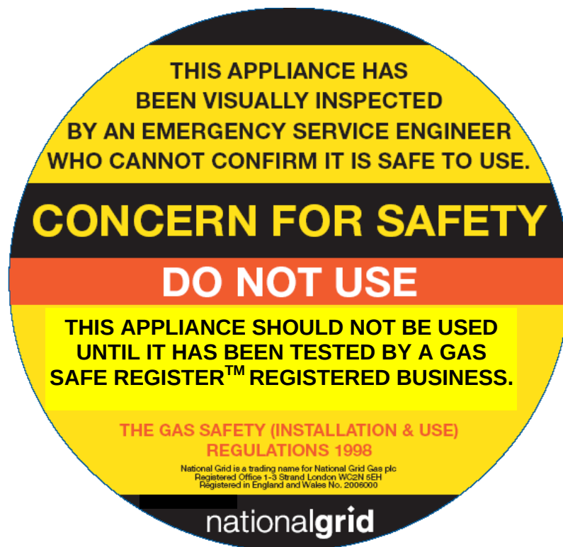
Figure 8 - Typical ESP 'Concern for Safety' label
