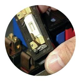
Checking a fuse carrier (base missing)
