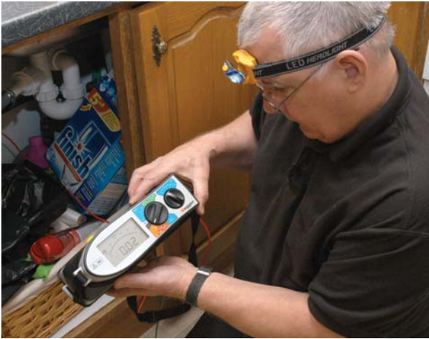
A continuity test being carried out
